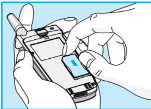
1. Remove the battery if attached.
